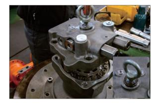
Assemble level gauge (44) into body (1).
