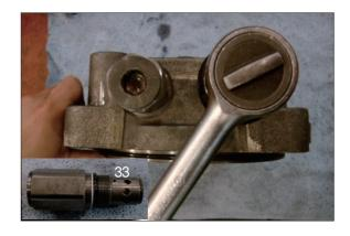
Assemble plug (37), plug (40, 41) into rear cover (21) with a L-wrench.\* Plug × 3 EA (PF1/4)
