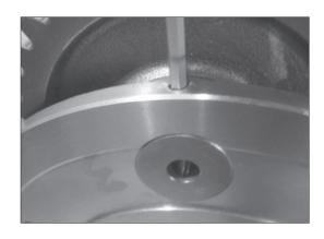
③ Remove planetary, thrust washer, No.1 pin, bearing from carrier.
