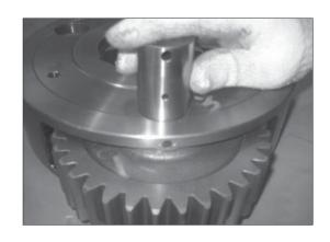
(3) Install No.1 pin into No.1 carrier where the holes for No.1 pin are to be in line with those of No.1 carrier, and then, install spring pins into the holes.
