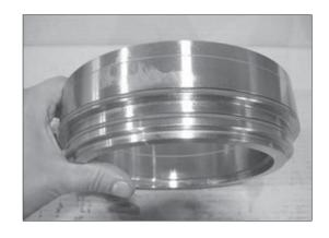
(24) Insert the parking piston into the casing and assemble it by using jig.
