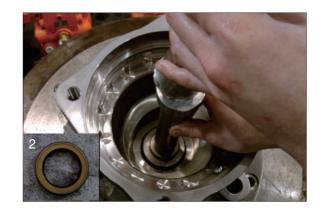
⑤ Insert above shaft sub into body (1) and assemble it with a steel stick.
