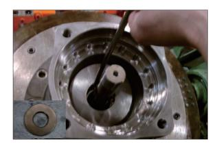
⑤ Using a plier jig, disassemble snap ring (4) from shaft (5).
