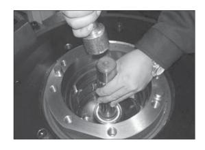
(15) Assemble the snap ring (11) into the casing (1) with the plier for retaining ring.
