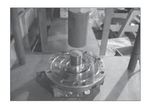
(6) Assemble the spring pin (32) and parallel pin (29) into rear cover (34) by using round bar or small hammer.
