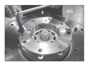
(25) Assemble the brake spring (30, 18EA) into the piston.
