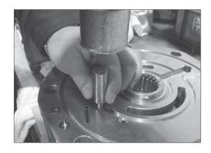
(7) Assemble the valve plate (28) into rear cover (34).Before assembling, apply some grease on
