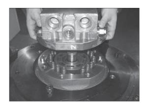
(4) Disassemble the brake spring (30, 18EA) from the piston.
