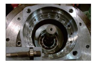
Fix snap ring (4) to shaft with a plier jig. Snap ring × 1 EA
