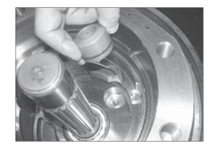
(18) Apply a little grease on the steel ball (15) and assemble it into the swash plate (17).
