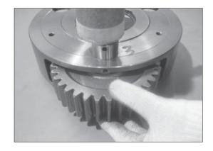
(4) Caulk carrier holes as shown on the picture.
