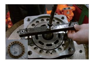
⑤ Disassemble respectively cylinder block assy, friction plate (15), plate (16) from body (1).
