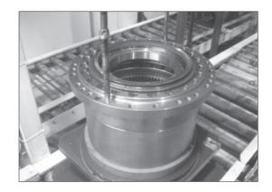
③ As the ring gear is adhered to housing assy, disassemble housing assy and ring gear by lightly hammering slantwise upward using sharpen punch inserted between the housing assy and ring gear.
