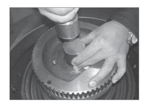
(11) Assemble the thrust plate (4) into the casing (1).
