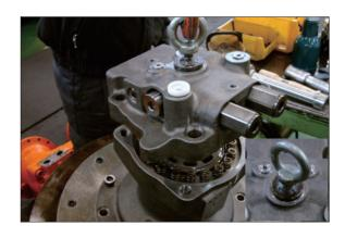
① Using a jig, disassemble break piston (17) from body (1).
