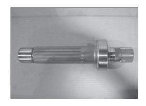
(14) Assemble the heat-fitted shaft (8) into casing (1).
