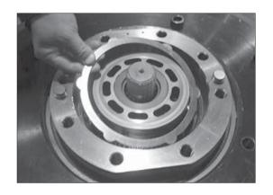
(23) Apply some grease on the D-ring and assemble it parking piston.
