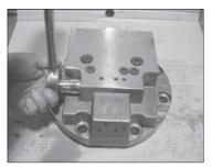
(21) Disassemble the plug (60) from the rear cover.
