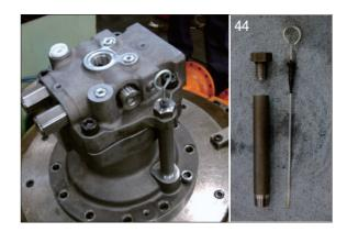
① Assemble time delay valve assy (35) into rear cover (21) with a wrench bolt (36).
