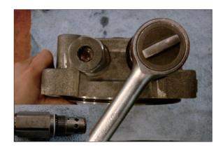
③ After disassembling plug with a L-wrench from rear cover (21), disassemble respectively back up ring, O-ring, O-ring, spring, anti-inversion valve assy (34)
