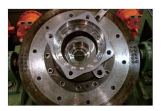
④ Using a compressing tool and steel stick, assemble oil seal (2) into body (1).
