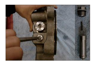
① Disassemble make up check valve assy with a torque wrench from rear cover (21).
