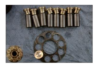
② Disassemble ball guide (12) from cylinder block (10).
