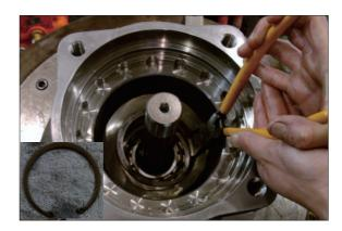
⑥ Disassemble shaft assy from body (1).
