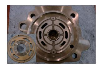
② Using a torque wrench, disassemble relief valve assy (33) 2 set from rear cover (21).
