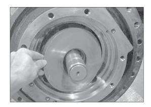
(20) Assemble the spring (19), ball guide (20), retainer plate (21) and piston assy (22) into cylinder block (18) in order.
