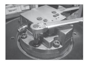
(3) Separate the casing (1) and rear cover (34).
